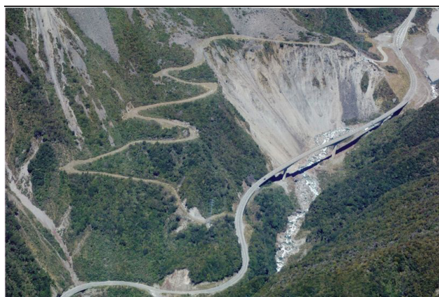
Figure 8.6. The Otira Viaduct, which bypasses the original, zig-zag road, in Arthurs Pass, Canterbury (Bell, 1999)
