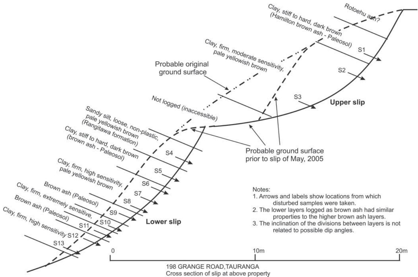
Figure 2. Cross section of the slope at 198 Grange Road, Tauranga.
