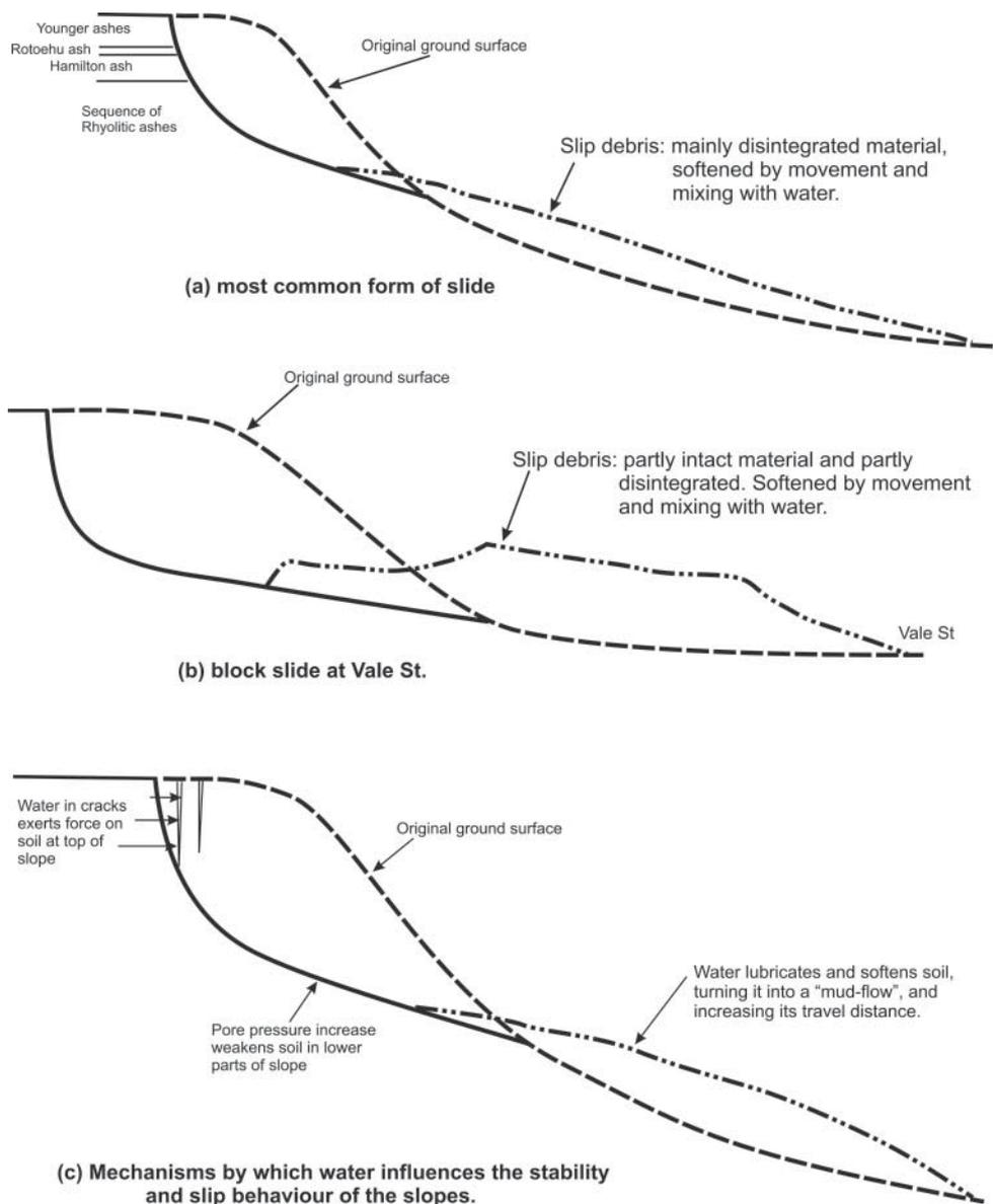
Figure 1. Forms of the slope failures.
