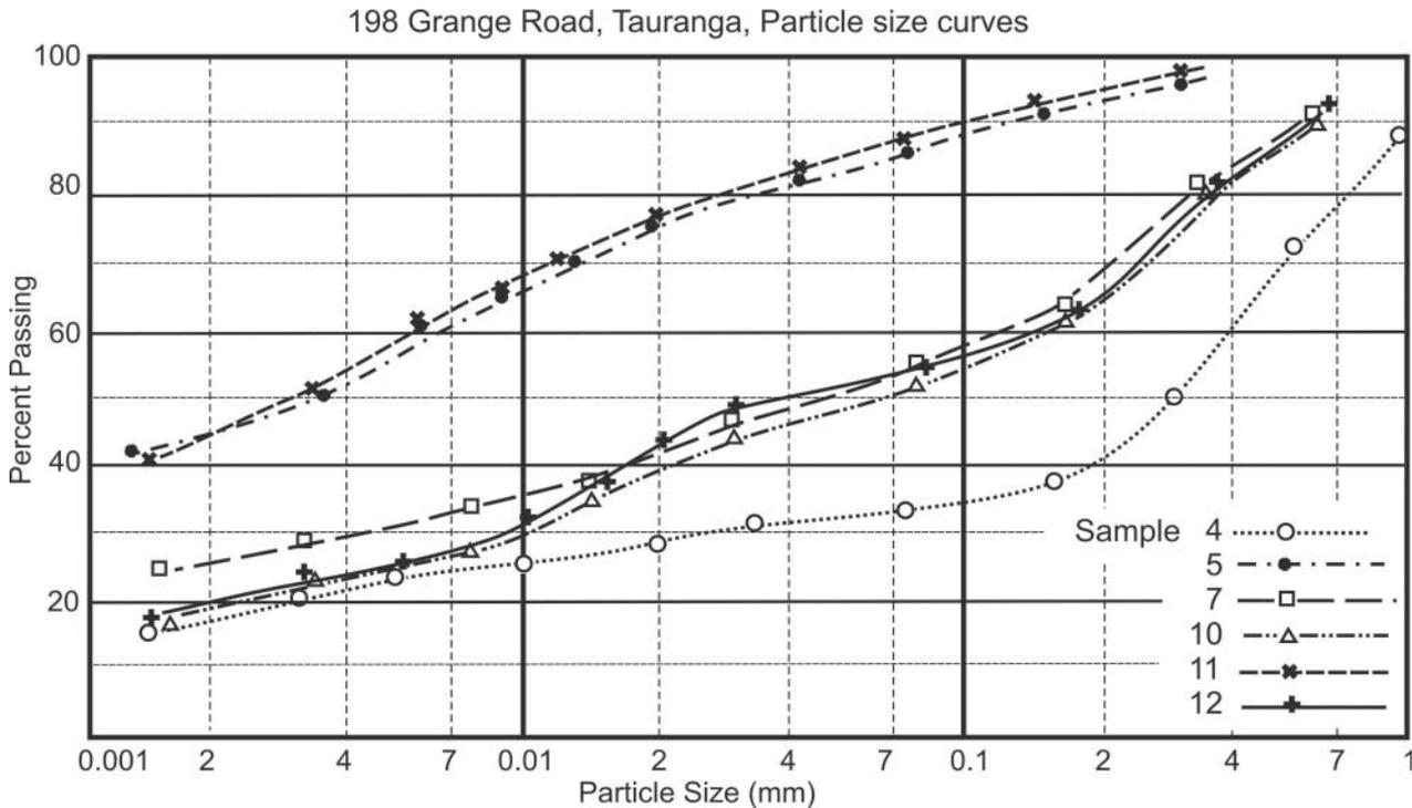
Figure 5. Particle size curves from four samples.
