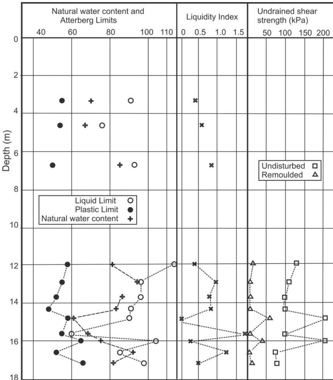
Figure 4. Results of tests on disturbed samples, plotted against depth.
