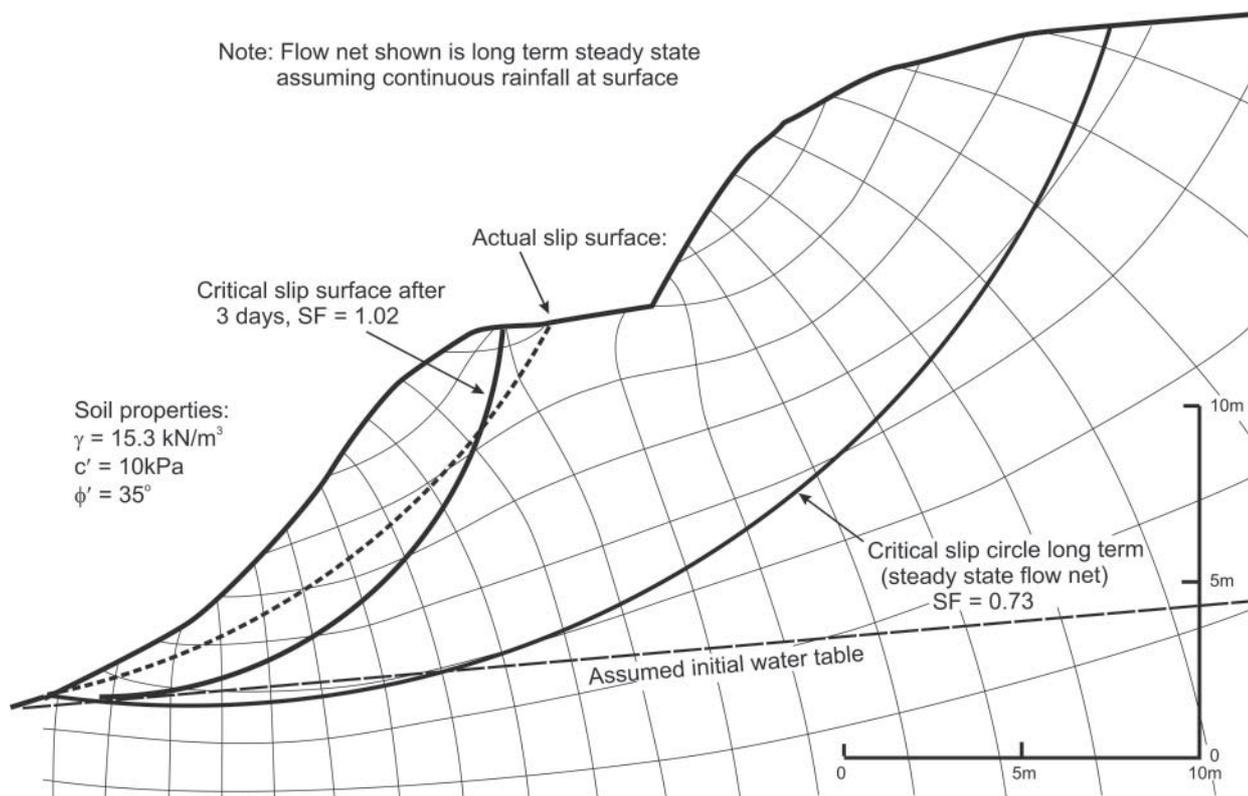
Figure 6. Slope cross section with flow net and failure surfaces.
